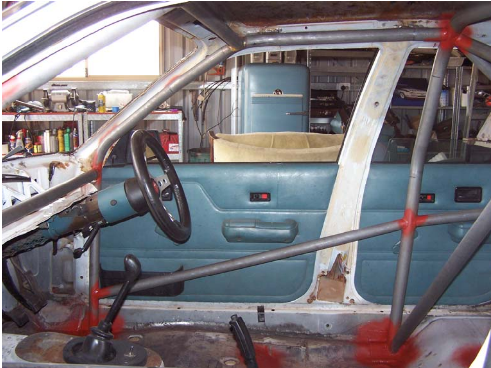
Interior with new roll cage. Welds undercoated.
